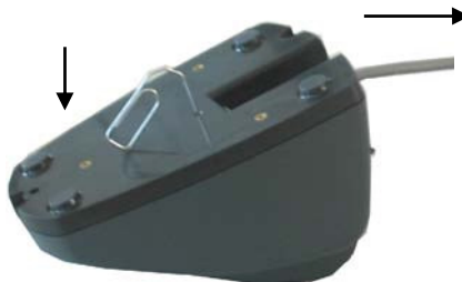
Disconnecting the Cable
