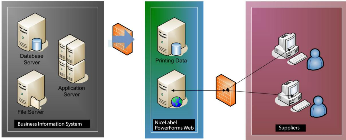
Figure 1: NiceLabel PowerForms Web Architecture
