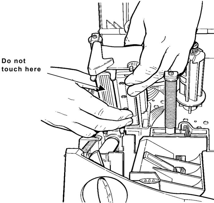
**Note:** Make sure the printhead cable does not touch the ribbon roll.
