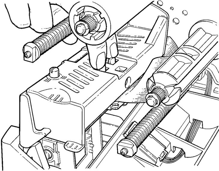
5. Lift the printhead assembly using the printhead tab and push back until the printhead assembly clicks into place.
